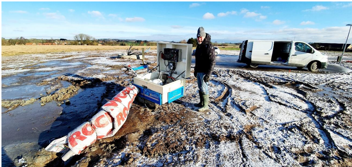
Figure 4. VIAs thermal response test equipment and laboratory chief Hans Erik Hansen. The equipment box contains a water circuit, circulation pump, 9 kW water heater and a Kamstrup Multical 801 energy meter. A circuit breaker panel ensures safe operation. The insulation of the connecting pipes minimizes heat loss to the atmosphere during the test.
